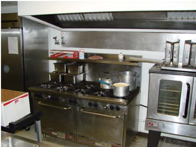
091_MI_1: Kitchen - Southbend 10-burner gas stove with double ovens.
